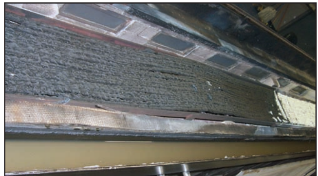
A before and after view of plenum cable being tested to see if it meets flammability specifications.
