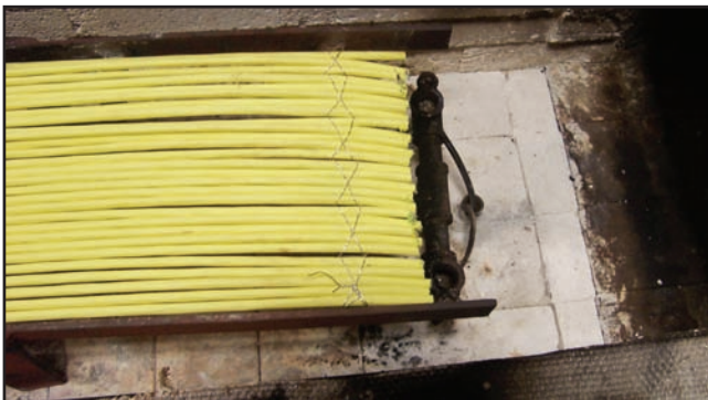
A before and after view of plenum cable being tested to see if it meets flammability specifications.
